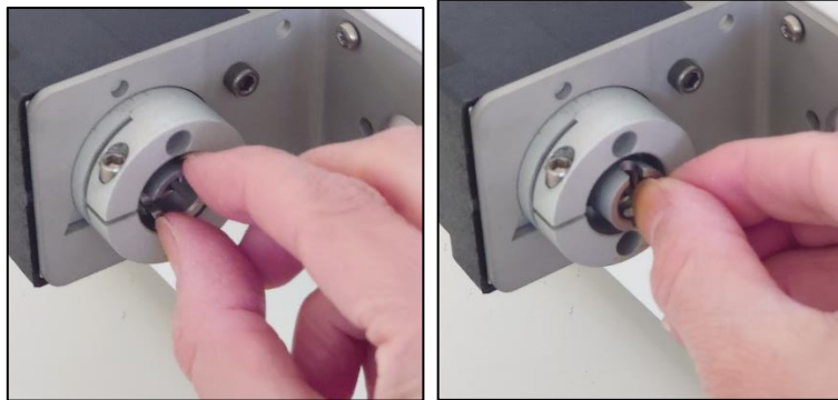
Figure 8 Changing the valve connection orientation in the valve clamp ring.
