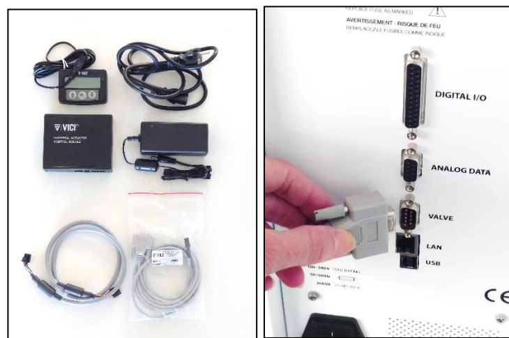
Figure 10 Cables from the valve kit and connection to the DECADE backpanel.
