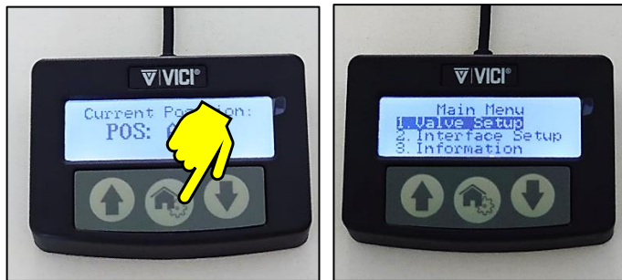
Figure 14 Open the Main Menu of the valve controller by holding the Home button pressed (about 5 sec) until the Main Menu opens
