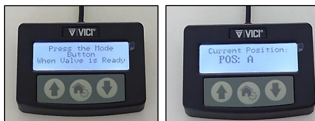
Figure 16 After automated initialization, the valve is defaulted to POS A
