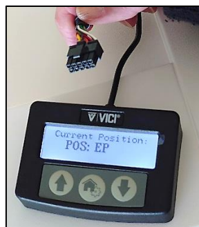
Figure 18 When switching the valve with a disconnected cable between the actuator and control module, the valve position becomes unknown, and the display shows POS: EP (error position).
