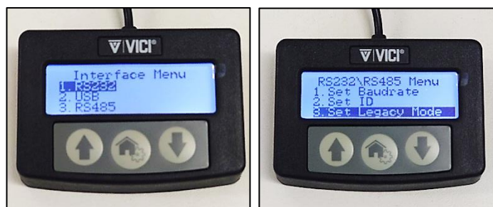
Figure 13 Set the RS232 communication to legacy mode
