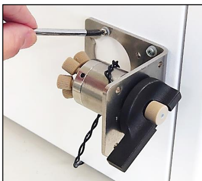
Figure 19 Attach the manual pre-mounted valve to the DECADE Elite/Lite
