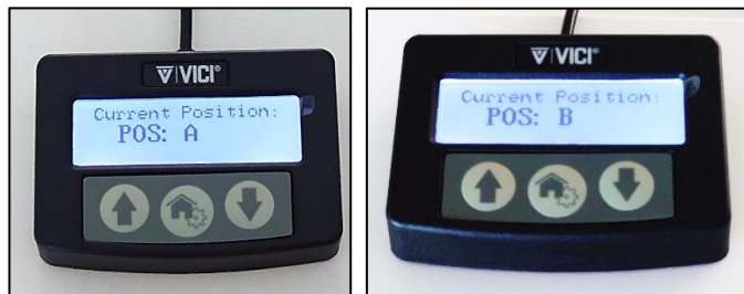
Figure 17 Alternately press the up and down buttons to switch between POS A and B on screen and thus initializing the valve.
